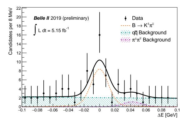
FIG. 8: Distribution of  $\Delta E$  for  $B^0 \to h^+ h'^ (h, h' = \pi \text{ or } K)$  candidates reconstructed in 5.15 fb<sup>-1</sup> of collision data. Shown are data points, superimposed on the result of a 1D unbinned extended maximum likelihood fit.
