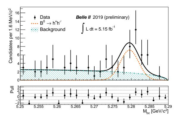
FIG. 3: Distribution of  $m_{bc}$  for  $B^0 \to h^+ h'^ (h, h' = \pi \text{ or } K)$  candidates reconstructed in 5.15 fb<sup>-1</sup> of collision data. Shown are data points, superimposed on the result of a 1D unbinned extended maximum likelihood fit, along with the pull distribution below.
