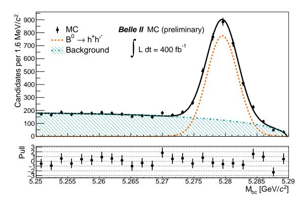
FIG. 1: Distribution of  $m_{bc}$  for  $B^0 \to h^+h'^ (h, h' = \pi \text{ or } K)$  candidates reconstructed in 400 fb<sup>-1</sup> of MC12b simulated data. Shown are data points, superimposed on the result of a 1D unbinned extended maximum likelihood fit, along with the pull distribution below.
