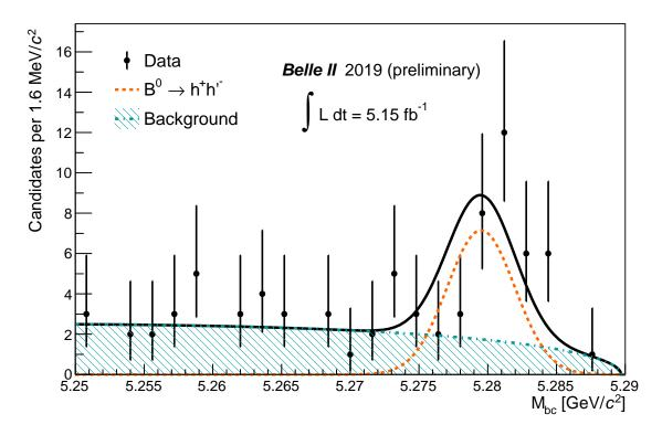
FIG. 4: Distribution of  $m_{bc}$  for  $B^0 \to h^+ h'^ (h, h' = \pi \text{ or } K)$  candidates reconstructed in 5.15 fb<sup>-1</sup> of collision data. Shown are data points, superimposed on the result of a 1D unbinned extended maximum likelihood fit.
