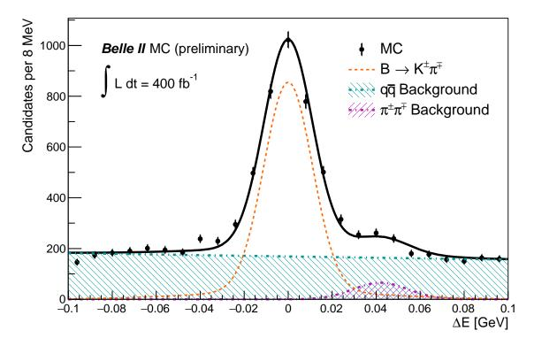
FIG. 6: Distribution of  $\Delta E$  for  $B^0 \to h^+ h'^ (h, h' = \pi \text{ or } K)$  candidates reconstructed in 400 fb<sup>-1</sup> of MC12b simulated data. Shown are data points, superimposed on the result of a 1D unbinned extended maximum likelihood fit.
